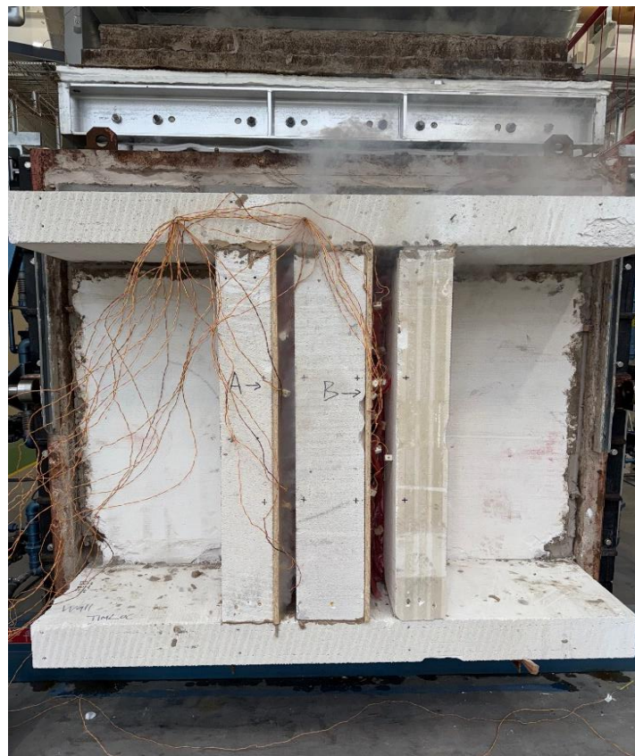
The unexposed face of the wall assembly after a test duration of 20 minutes
