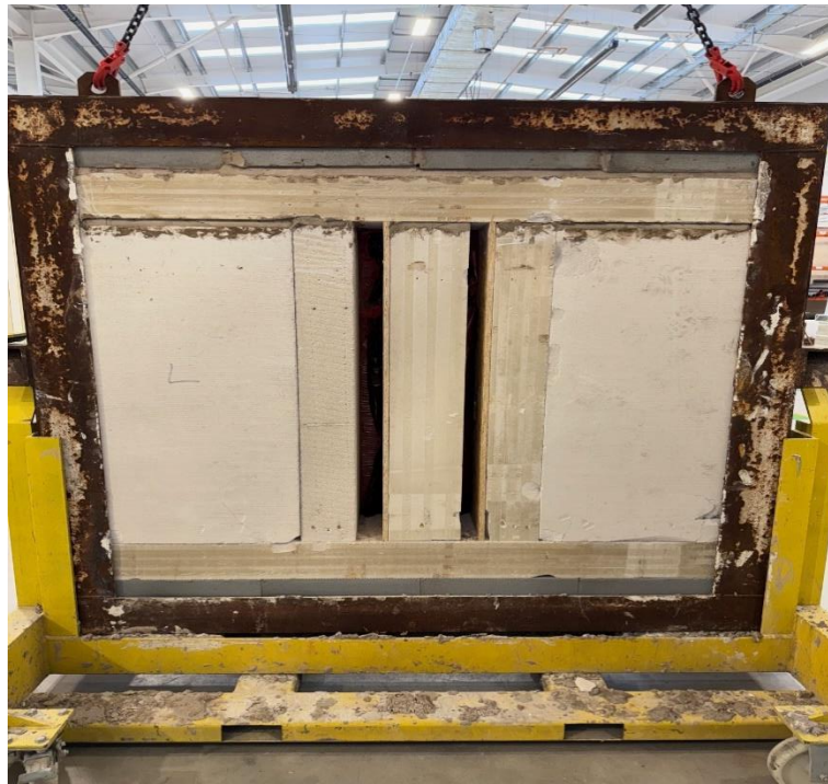
The exposed face of the wall assembly prior to testing
