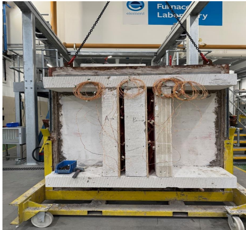
The unexposed face of the wall assembly prior to the start of the test
