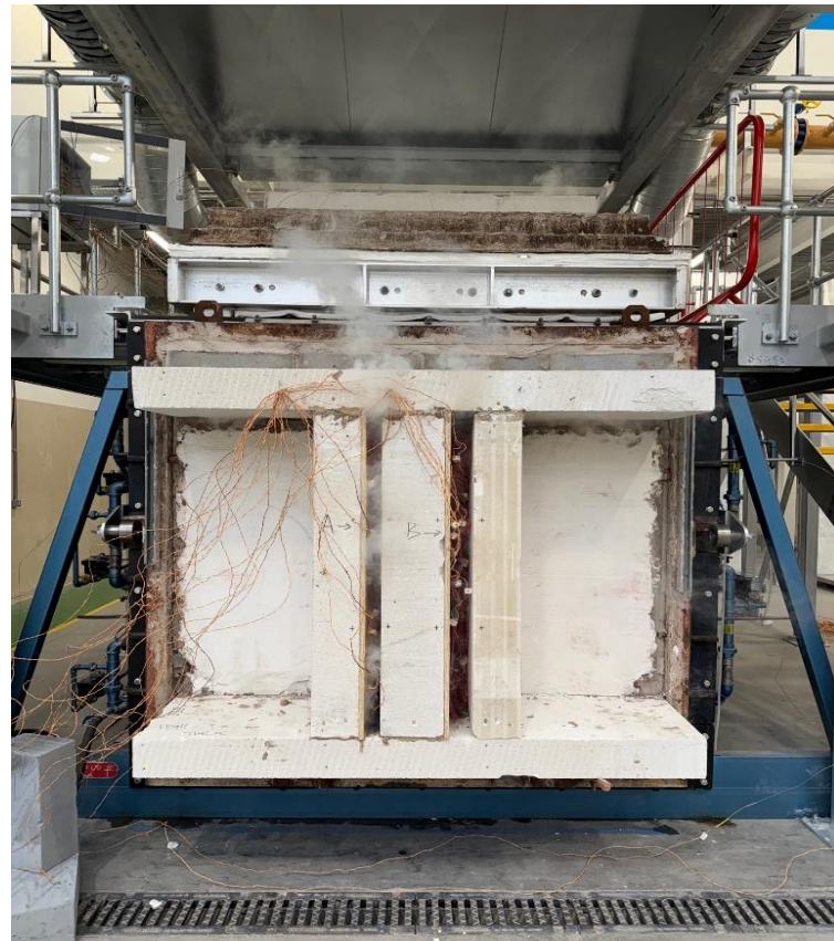
The unexposed face of the wall assembly after a test duration of 30 minutes
