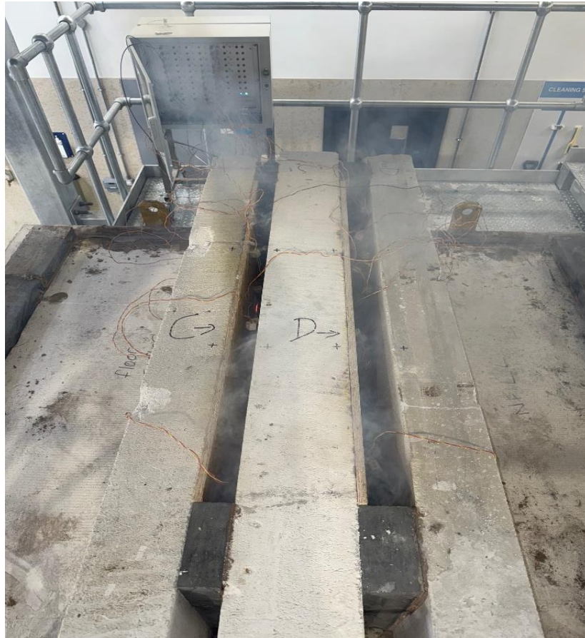
The unexposed face of the floor assembly after a test duration of 60 minutes
