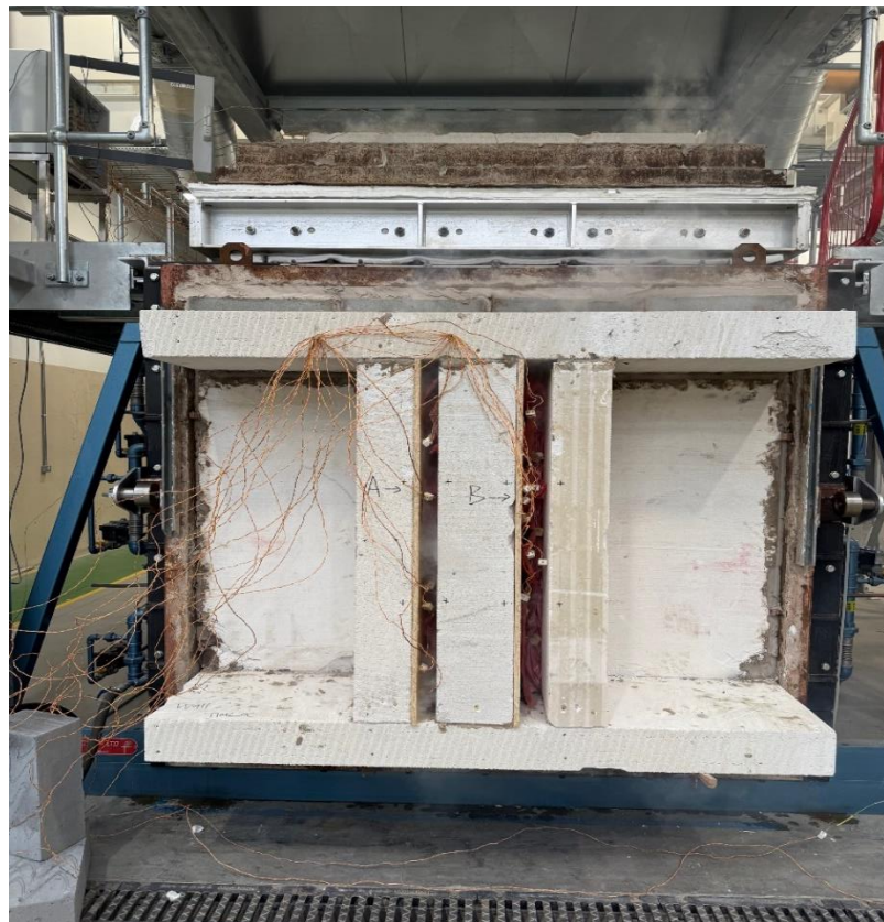
The unexposed face of the wall assembly after a test duration of 10 minutes
