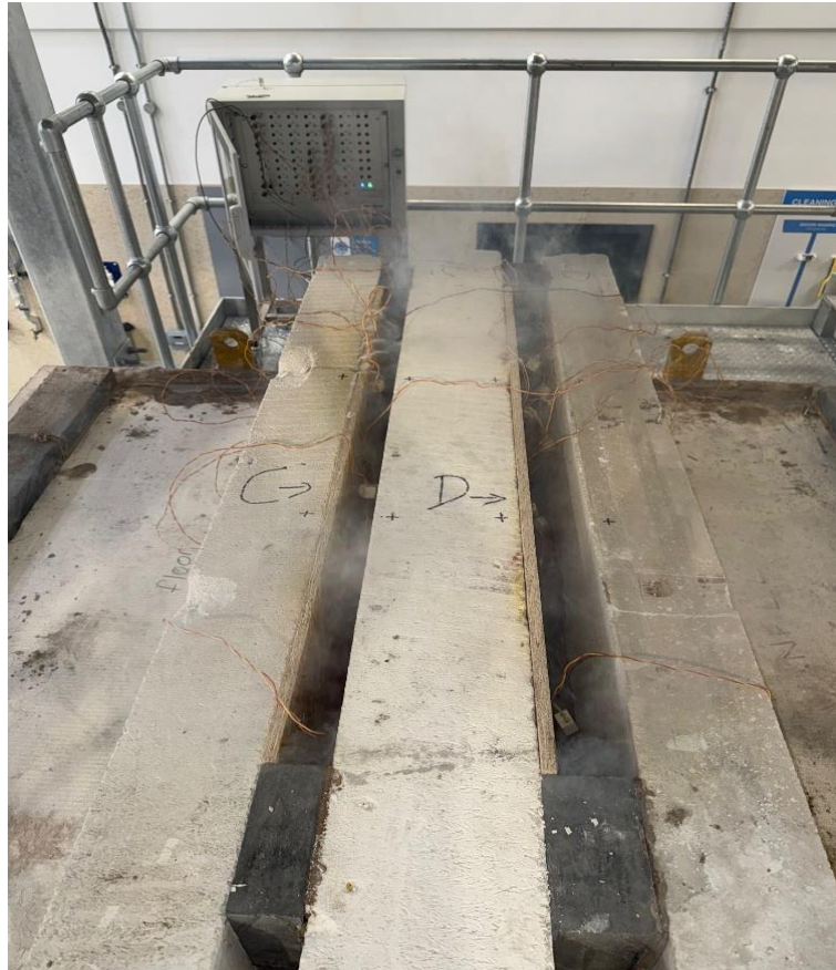
The unexposed face of the floor assembly after a test duration of 50 minutes
