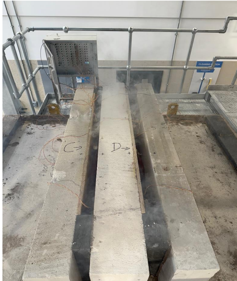
The unexposed face of the floor assembly after a test duration of 40 minutes
