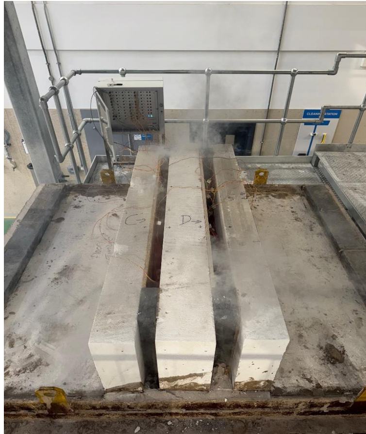
The unexposed face of the floor assembly after a test duration of 20 minutes
