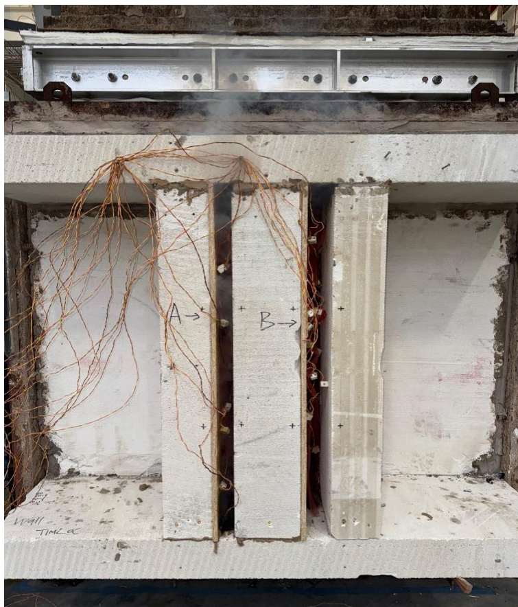
The unexposed face of the wall assembly after a test duration of 60 minutes
