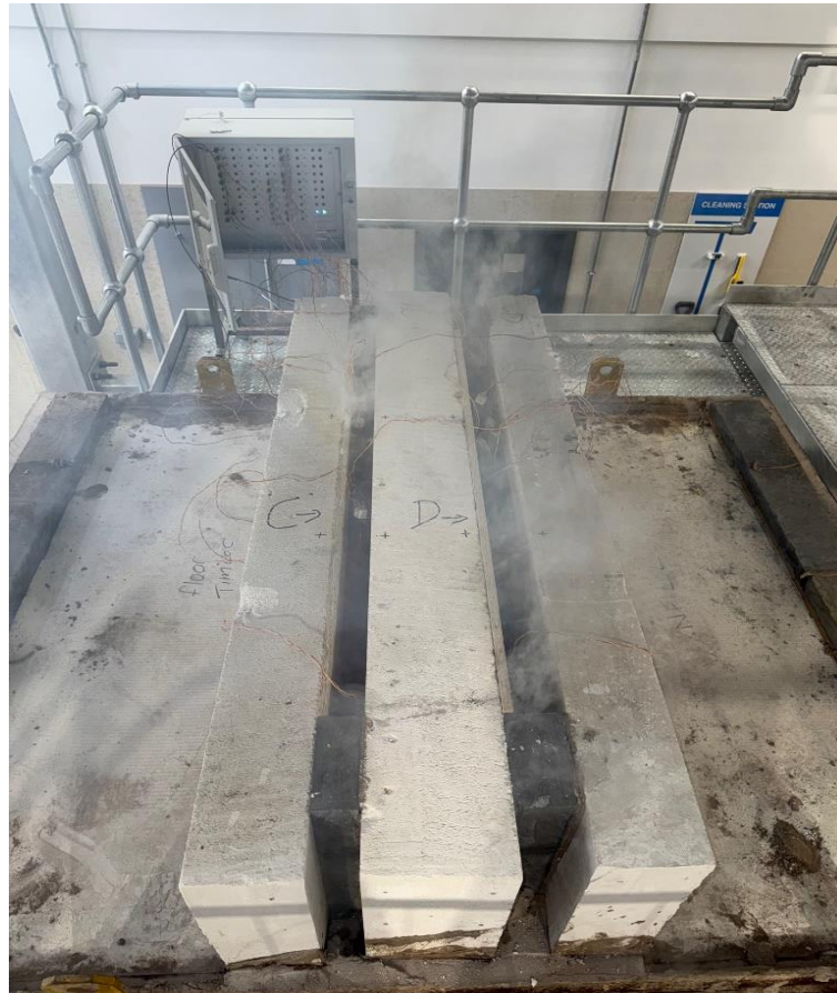
The unexposed face of the floor assembly after a test duration of 30 minutes
