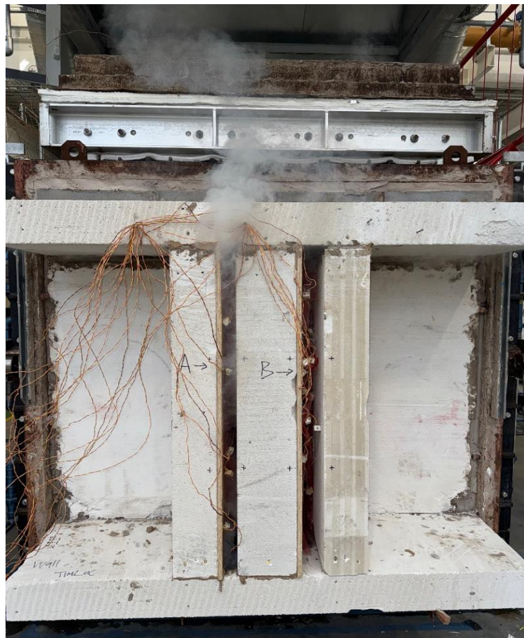
The unexposed face of the wall assembly after a test duration of 40 minutes
