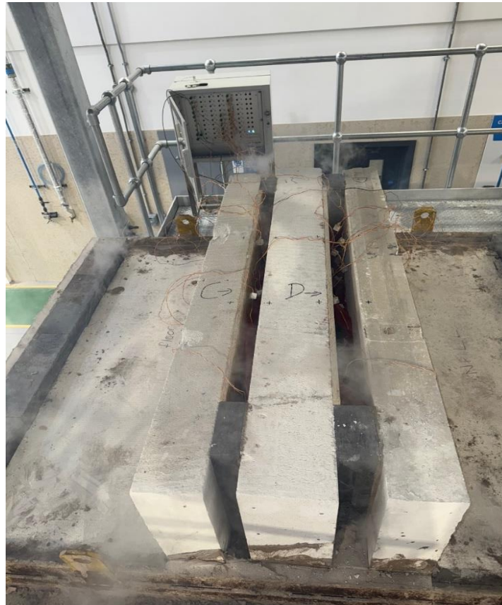
The unexposed face of the floor assembly after a test duration of 10 minutes
