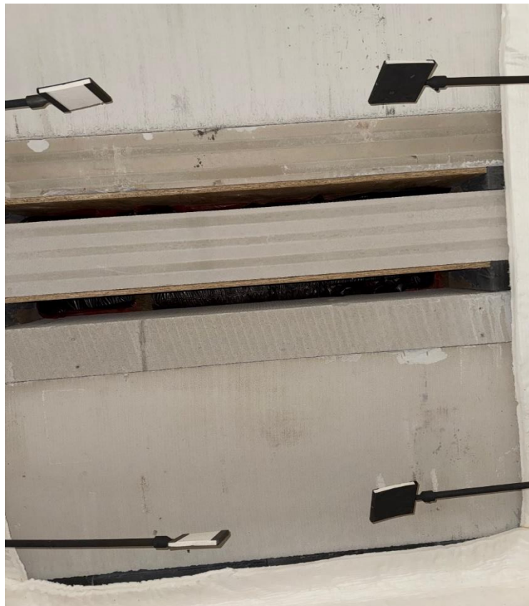
The exposed face of the floor assembly prior to testing
