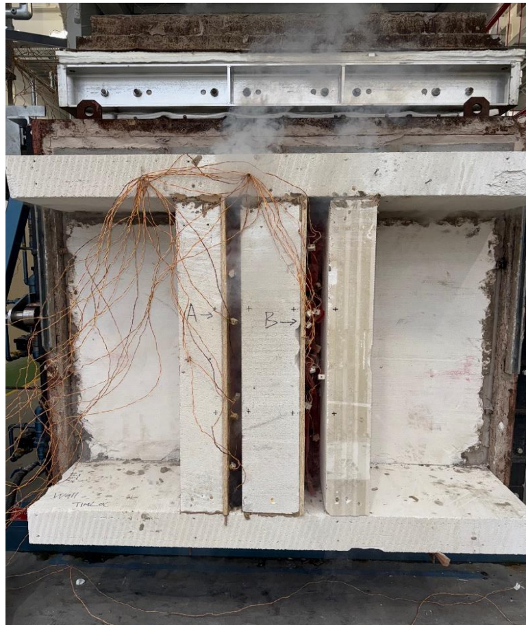
The unexposed face of the wall assembly after a test duration of 50 minutes
