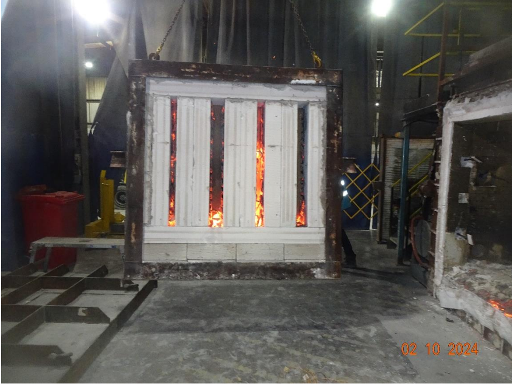
The unexposed face of the wall assembly immediately after the test duration
