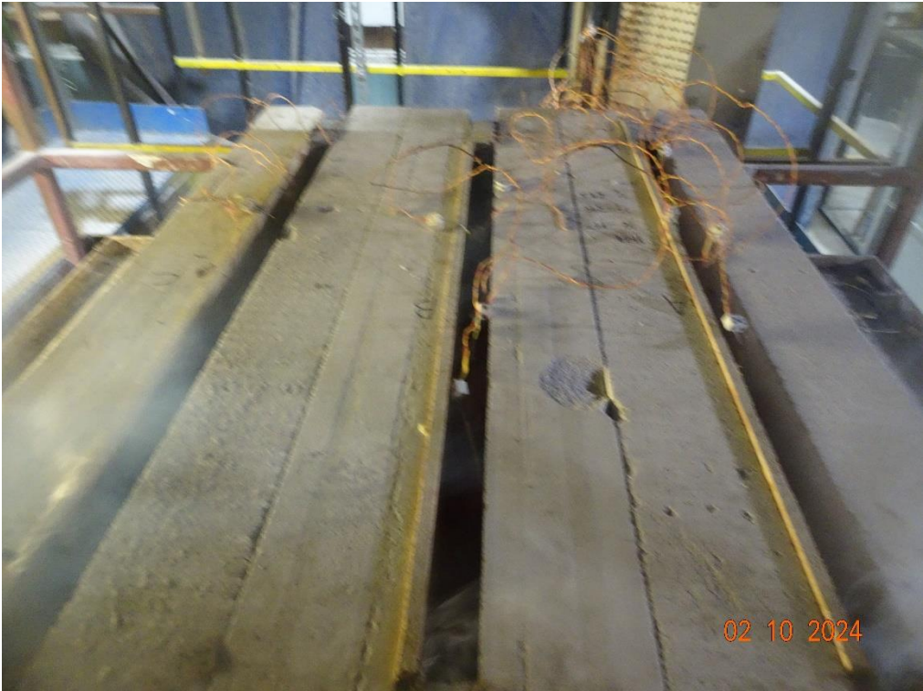
The unexposed face of the floor assembly after a test duration of 66 minutes
