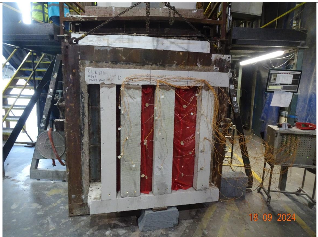
The unexposed face of the wall assembly prior to testing
