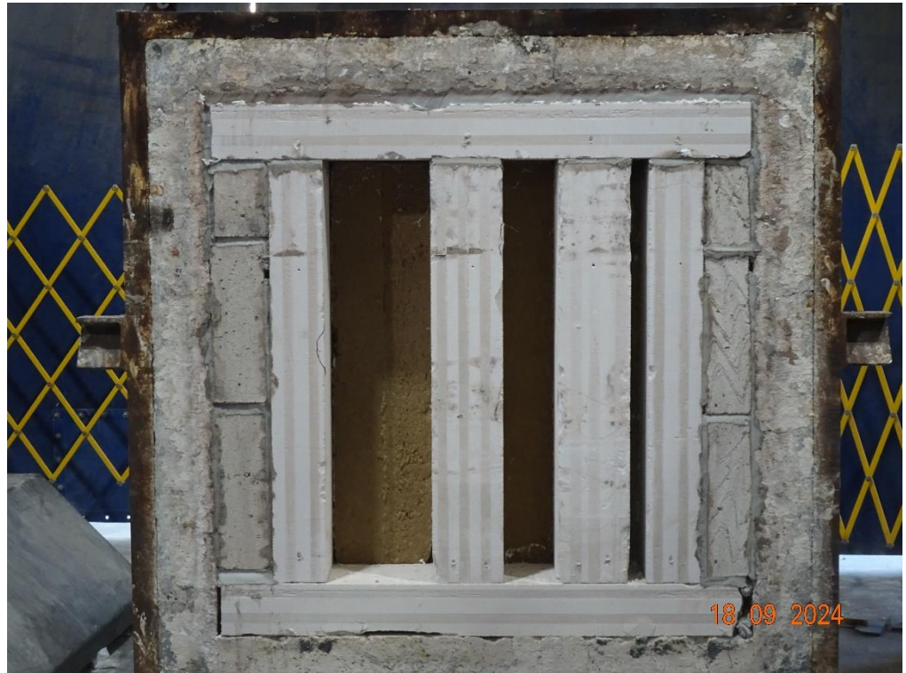
The exposed face of the wall assembly immediately after the test duration
