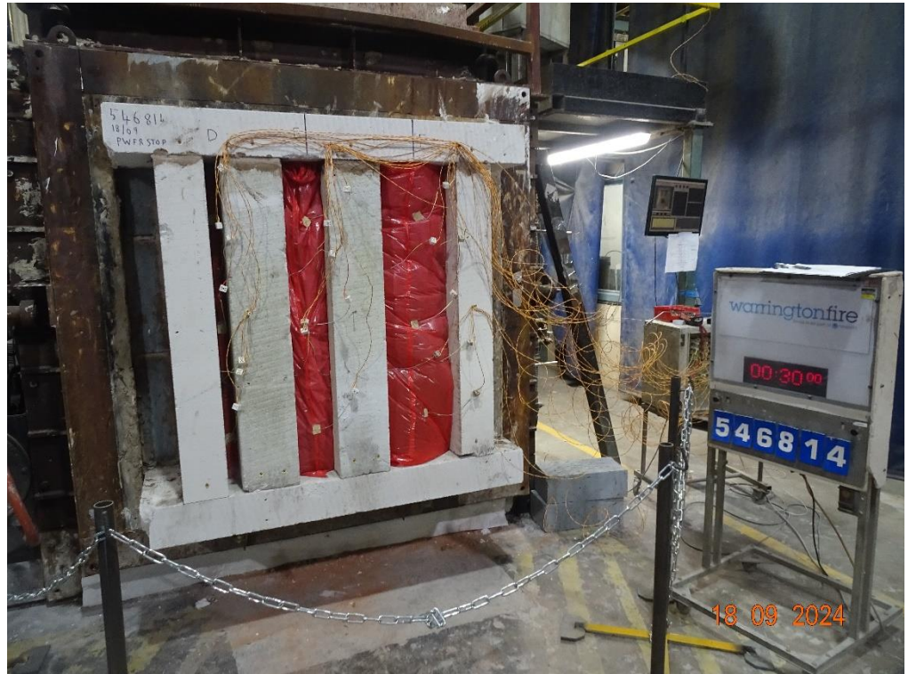
The unexposed face of the wall assembly after a test duration of 30 minutes
