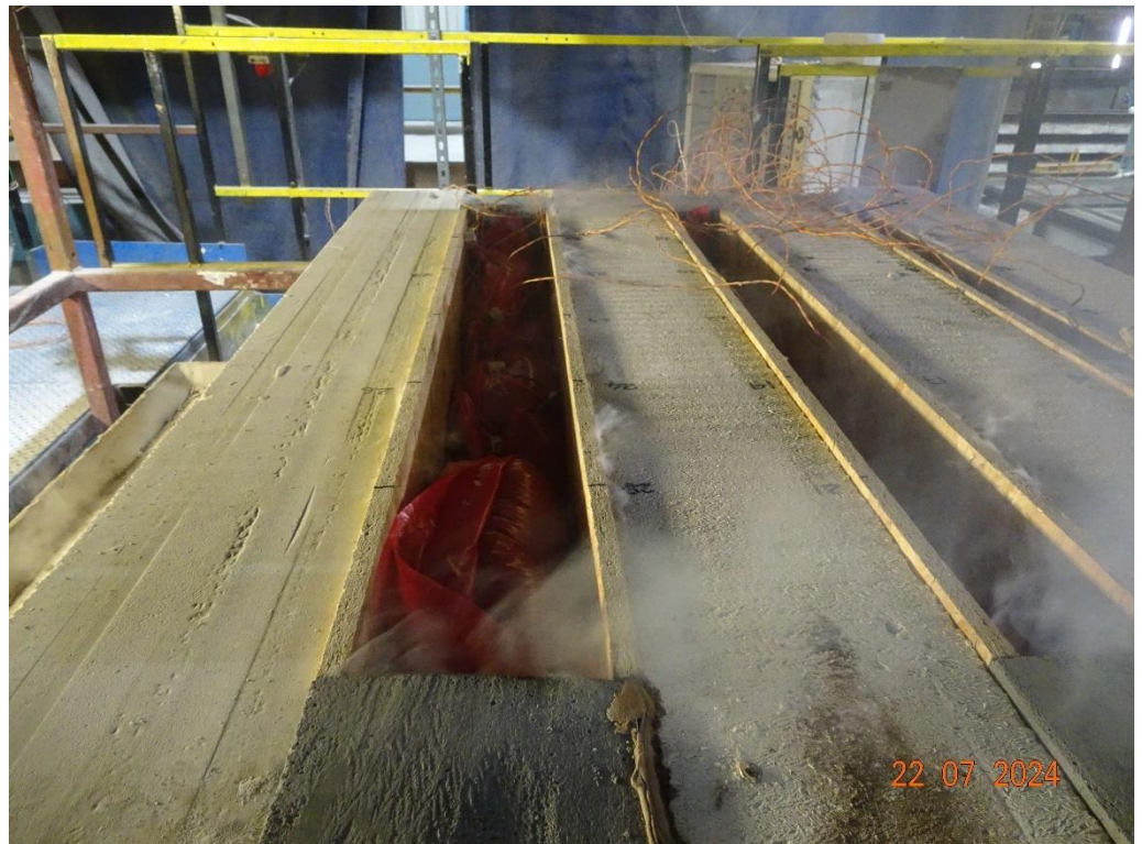
The exposed face of the floor assembly after a test duration of 60 minutes.
