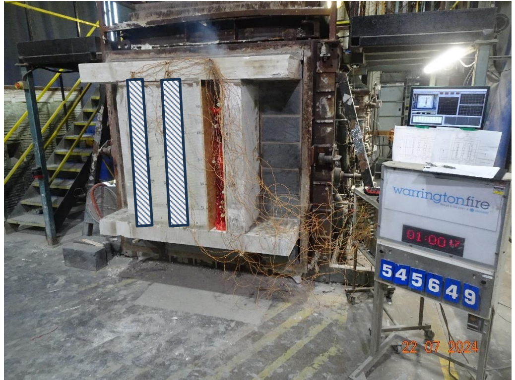
The exposed face of the wall assembly after a test duration of 60 minutes.
