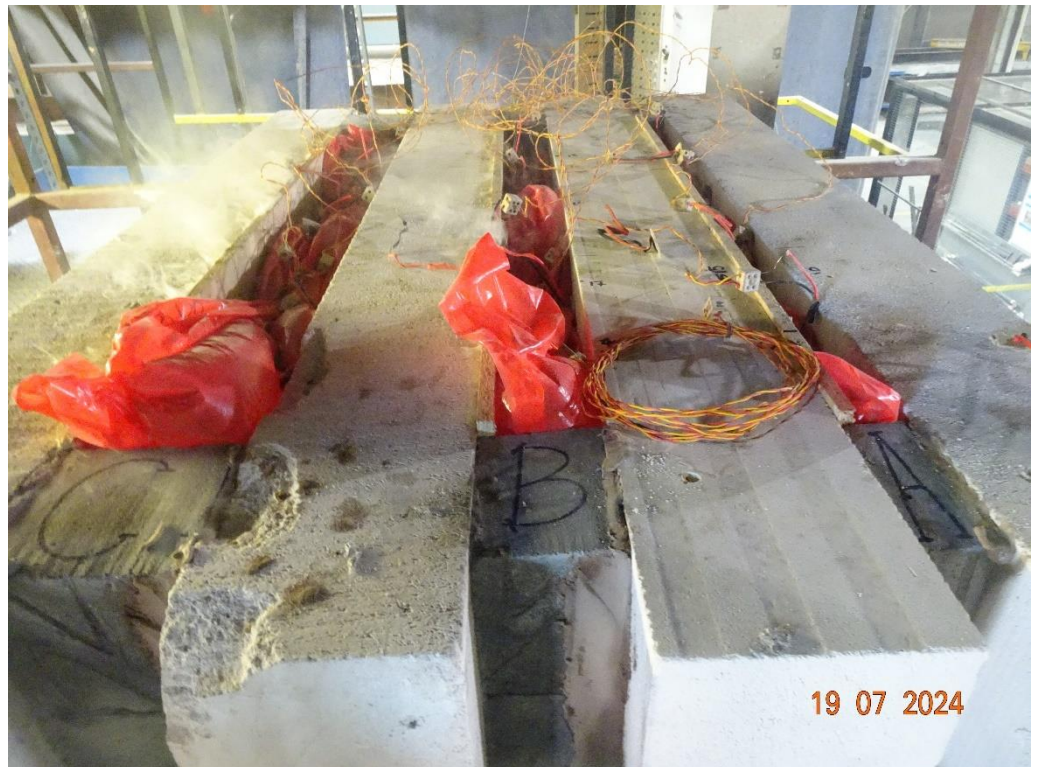
The unexposed face of the floor assembly after a test duration of 60 minutes
