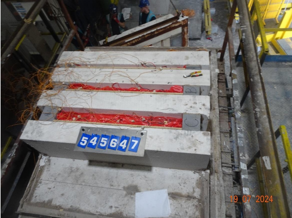
The unexposed face of the floor assembly prior to the start of the test
