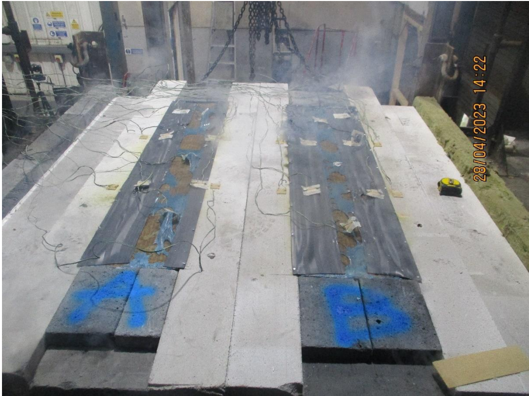
The unexposed horizontal face after a test duration of 20 minutes
