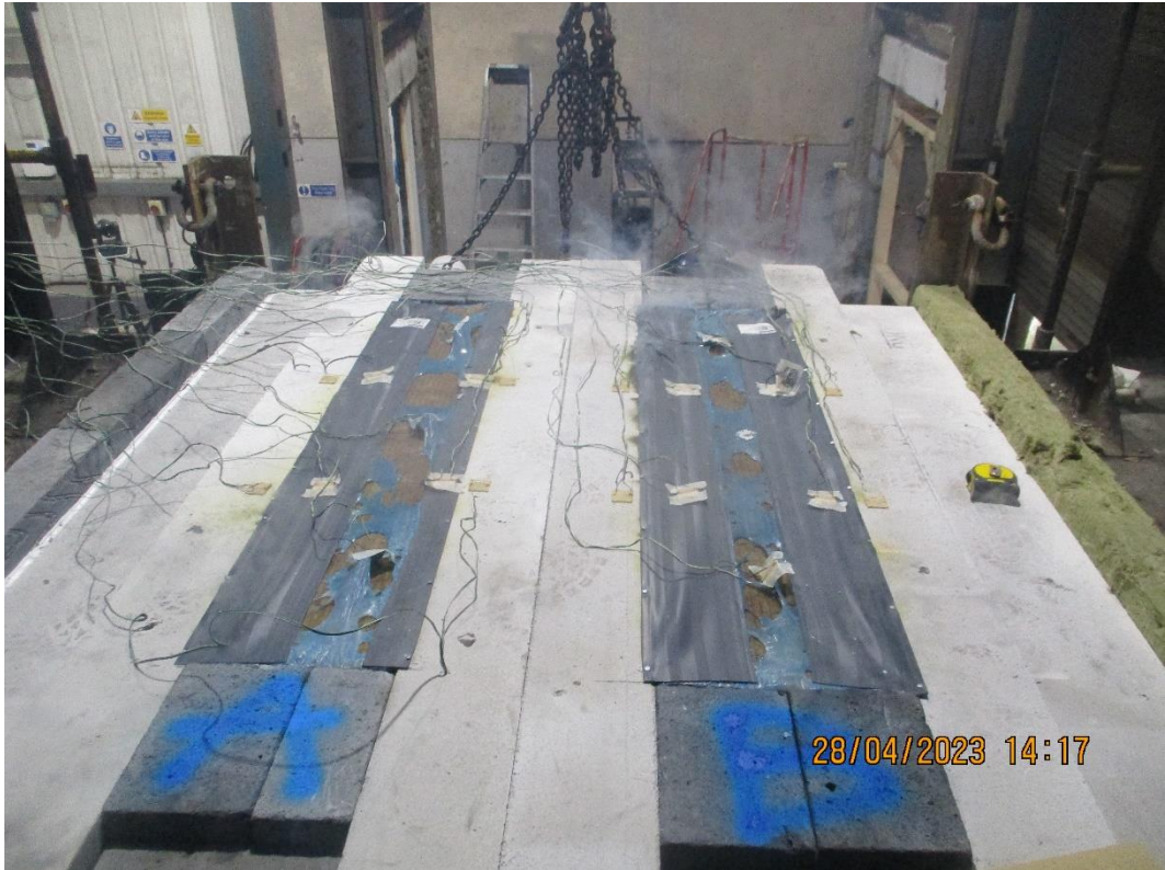
The unexposed horizontal face after a test duration of 15 minutes
