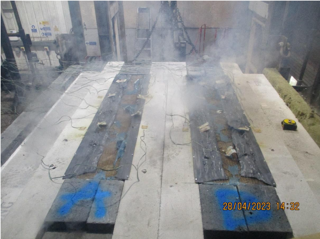
The unexposed horizontal face after a test duration of 30 minutes
