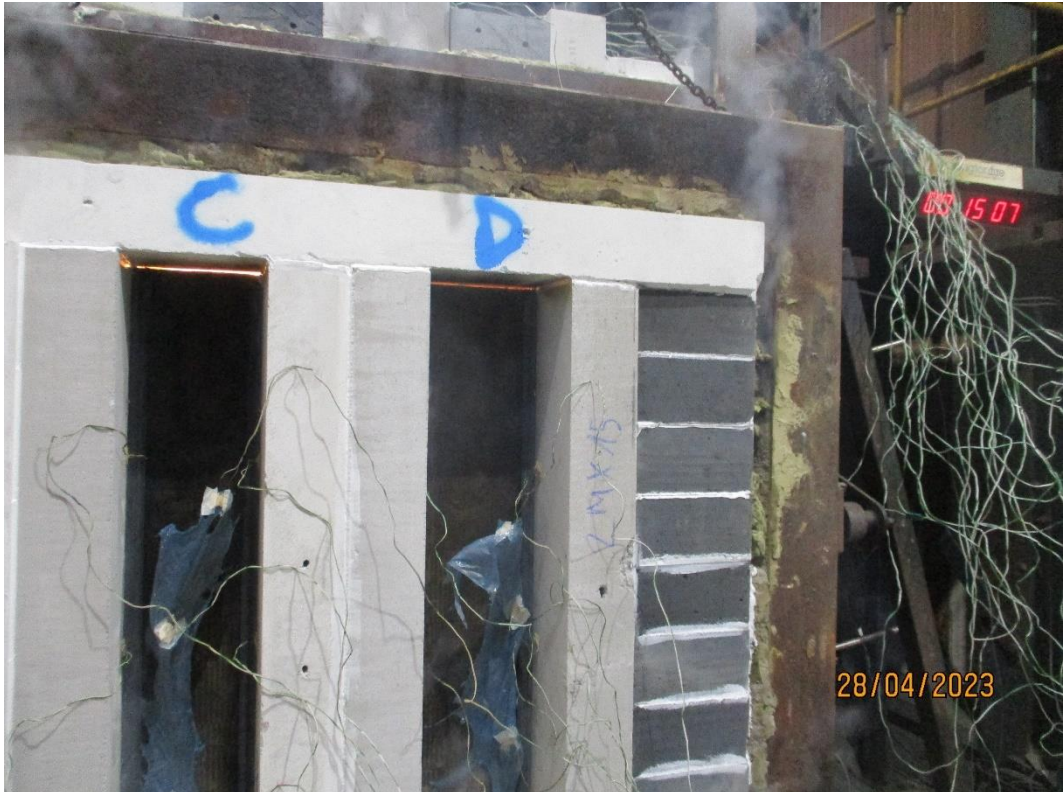
The unexposed vertical face after a test duration of 15 minutes 7 seconds
