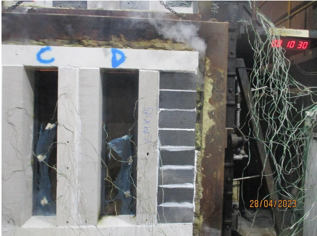
The unexposed vertical face after a test duration of 10 minutes 30 seconds
