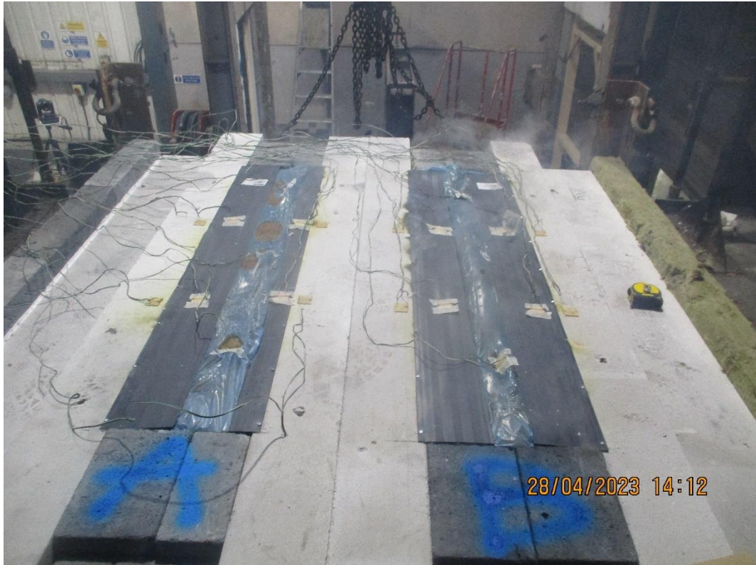
The unexposed horizontal face after a test duration of 10 minutes
