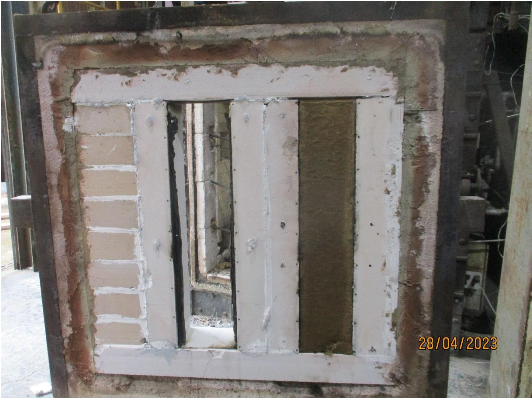
The exposed vertical face after the completion of the test
