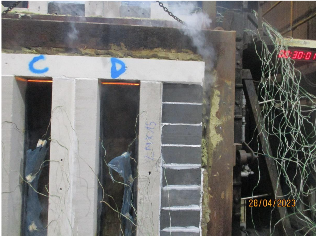
The unexposed vertical face after a test duration of 30 minutes 1 second
