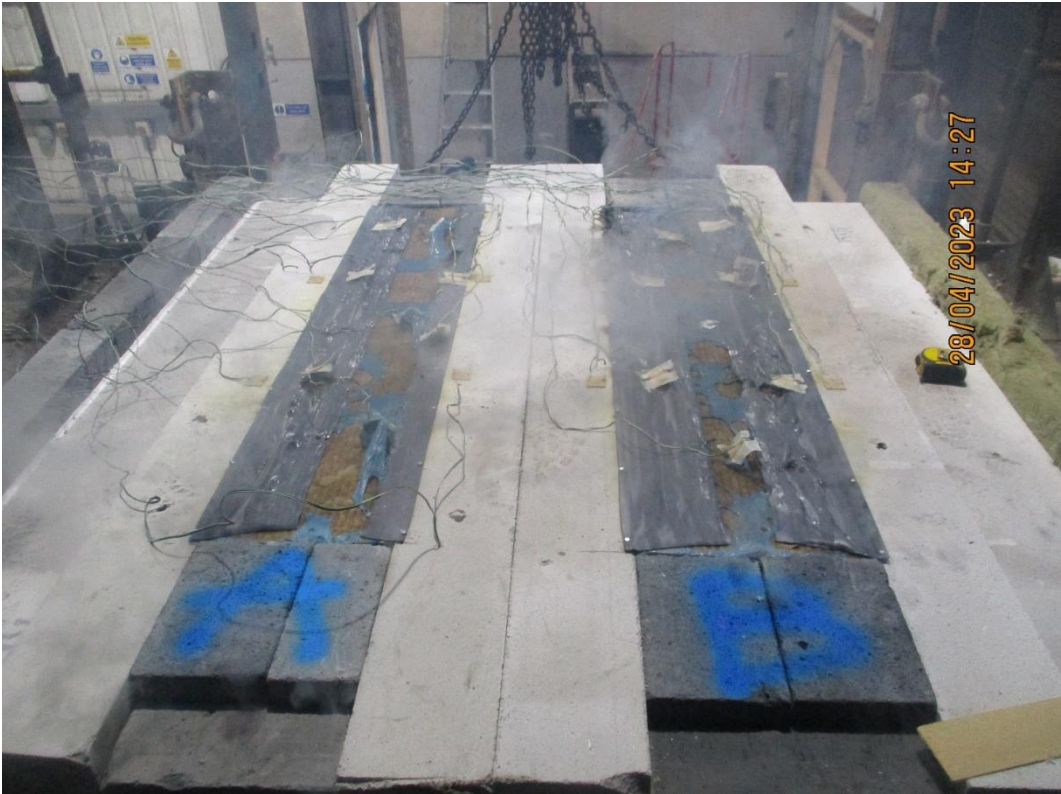
The unexposed horizontal face after a test duration of 25 minutes
