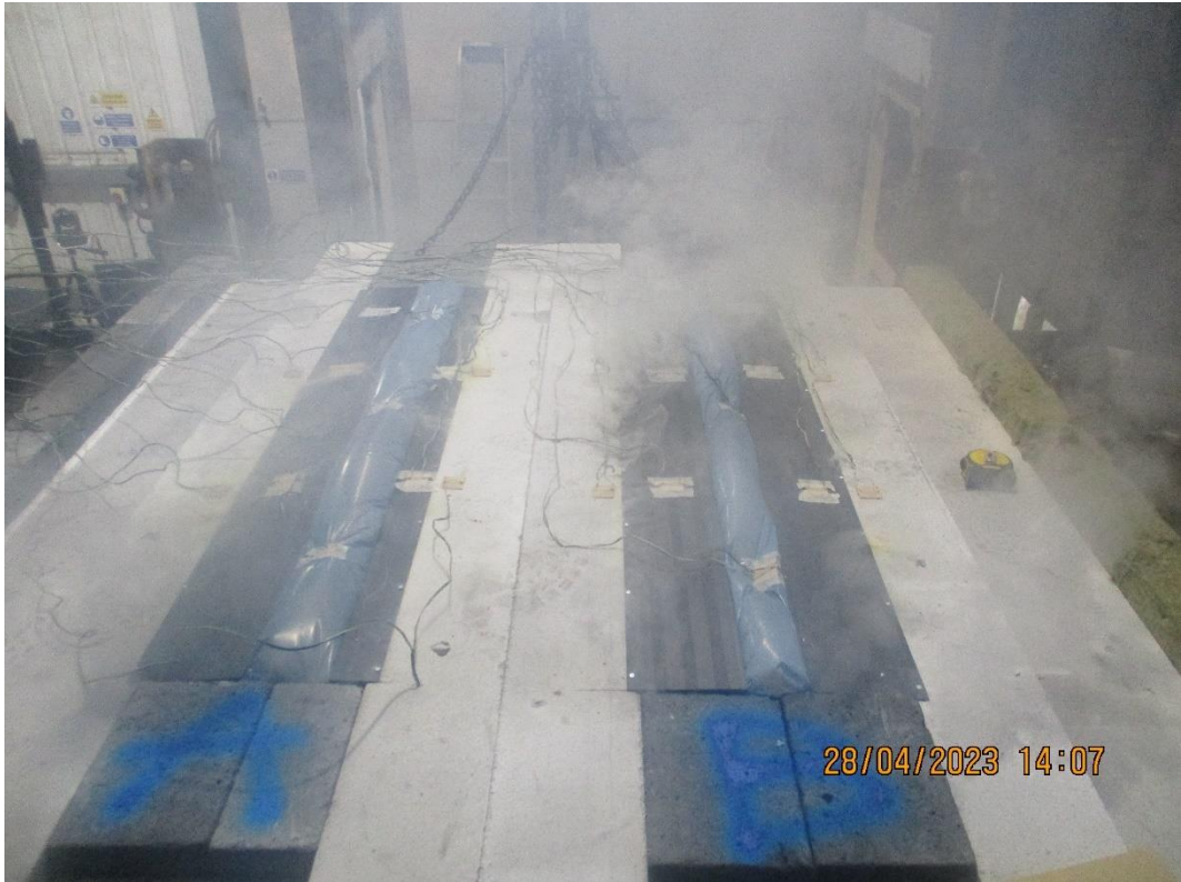
The unexposed horizontal face after a test duration of 5 minutes
