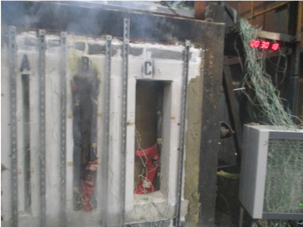
The unexposed face after a test duration of 30 minutes 18 seconds
