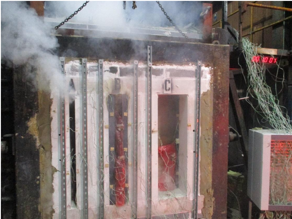
The unexposed face after a test duration of 10 minutes 1 second
