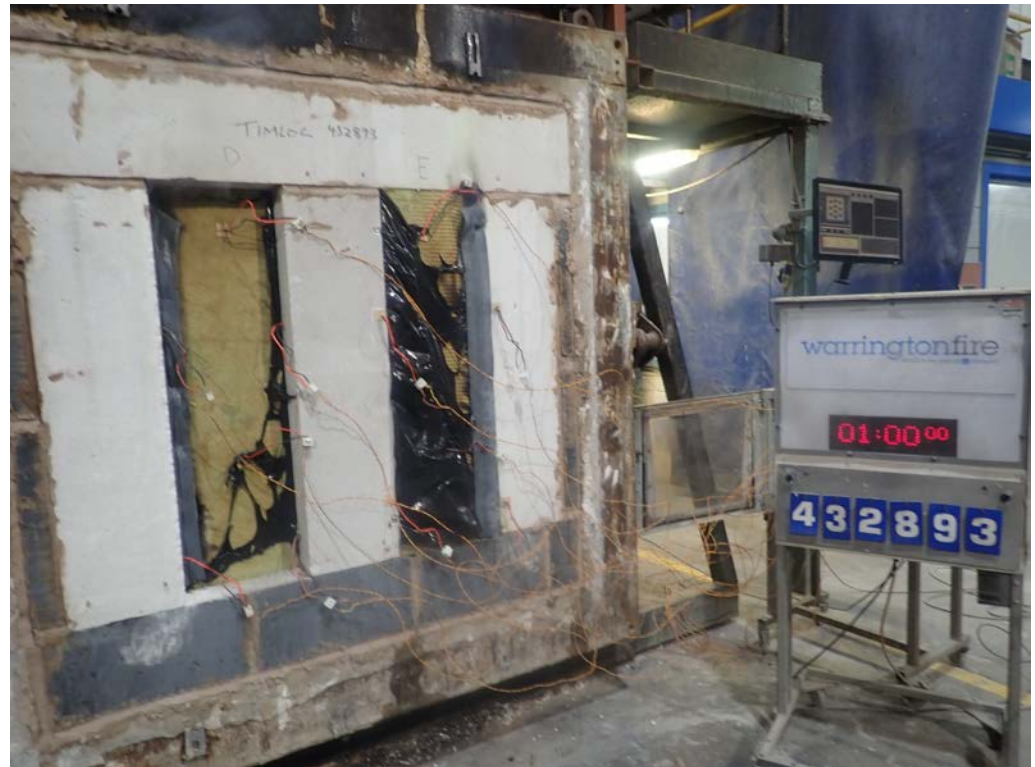
The unexposed face of the vertical assembly after a test duration of 60 minutes
