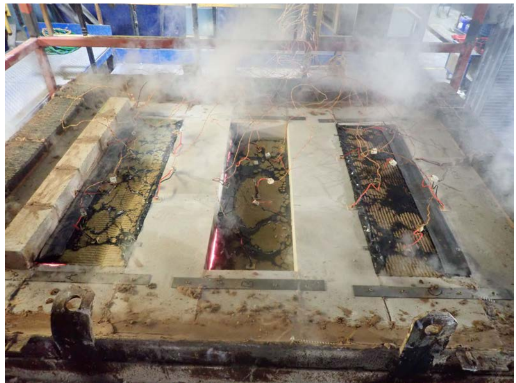
The unexposed face of the horizontal assembly after a test duration of 60 minutes
