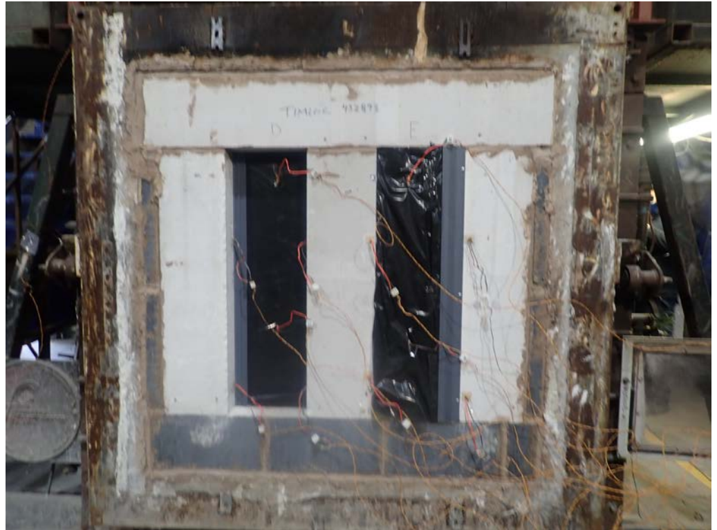
The unexposed face of the vertical assembly prior to the start of the test
