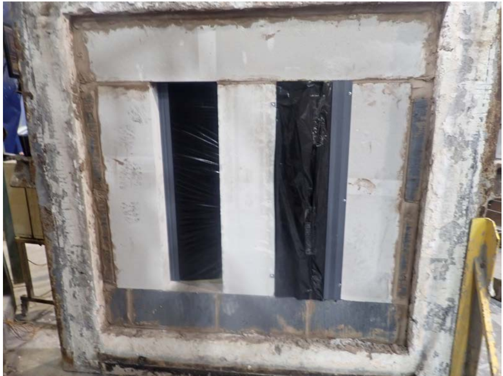
The exposed face of the vertical assembly prior to testing
