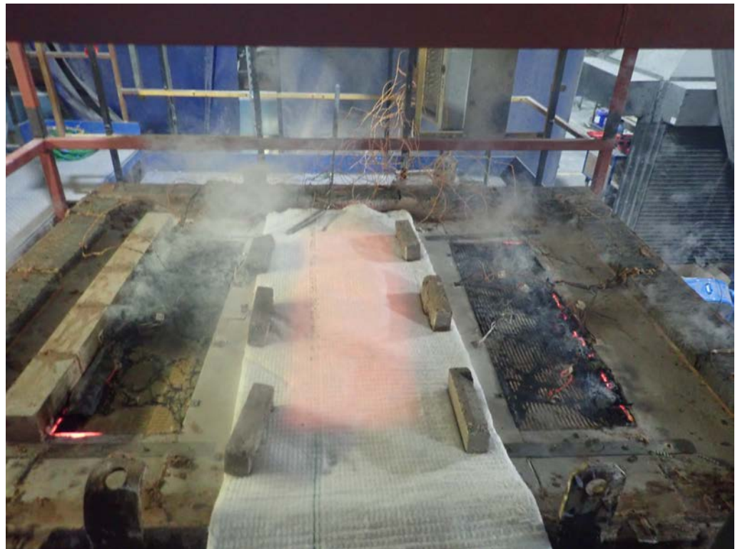
The unexposed face of the horizontal assembly after a test duration of 95 minutes
