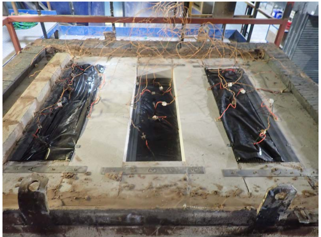
The unexposed face of the horizontal assembly prior to the start of the test
