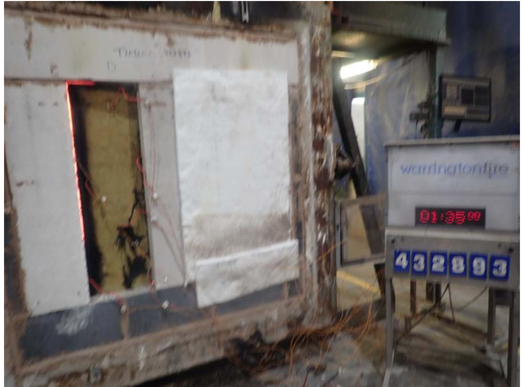
The unexposed face of the vertical assembly after a test duration of 95 minutes
