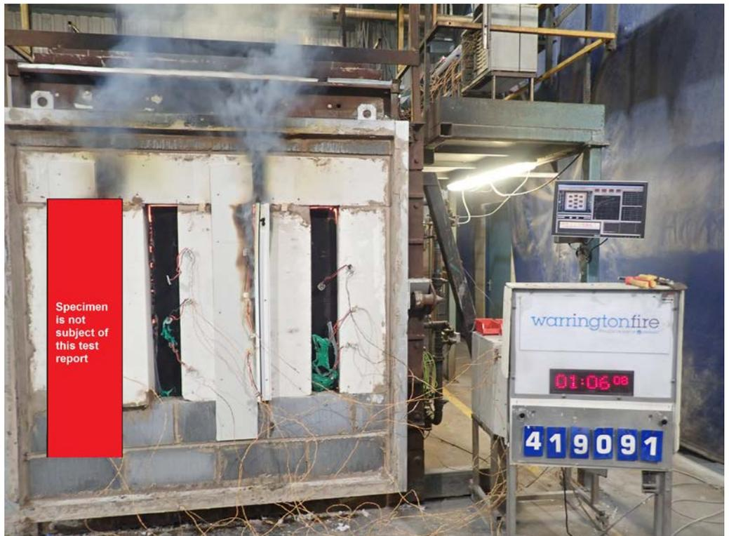
The unexposed face of the wall after 71 minutes of testing showing sustained flaming issues to Specimen G
