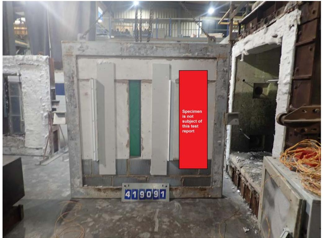
The unexposed face of the wall after 10 minutes of testing
