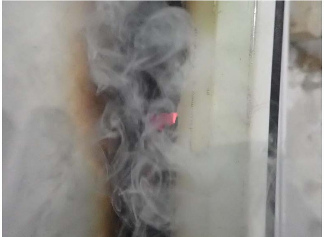
The unexposed face of the wall after 66 minutes of testing
