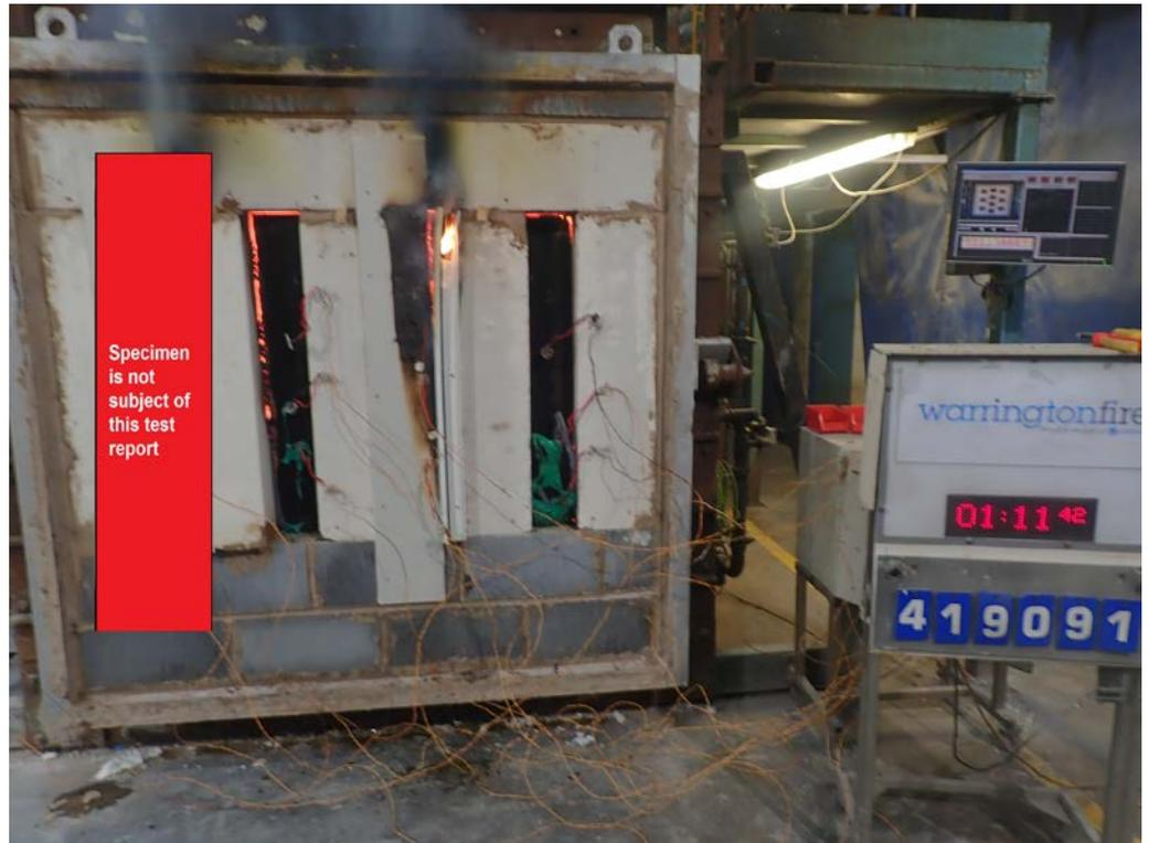
The unexposed face of the wall after 72 minutes of testing
