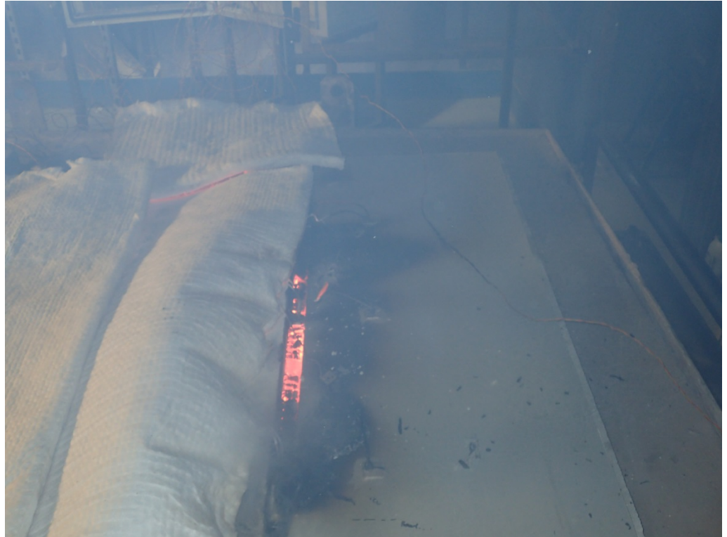
Integrity failure of Specimen F after a test duration of 53 minutes
