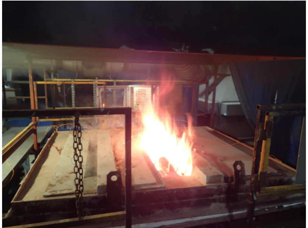
Specimen E falls away after a test duration of 41 minutes
