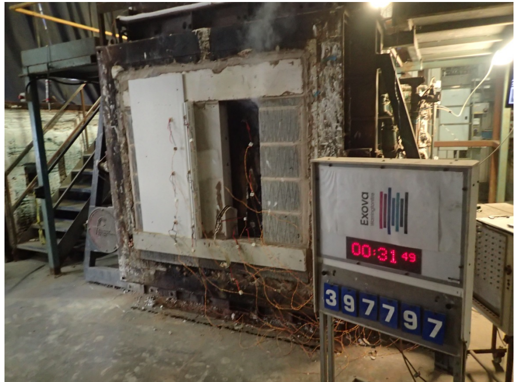
The unexposed face of the wall assembly after a test duration of 31 minutes
