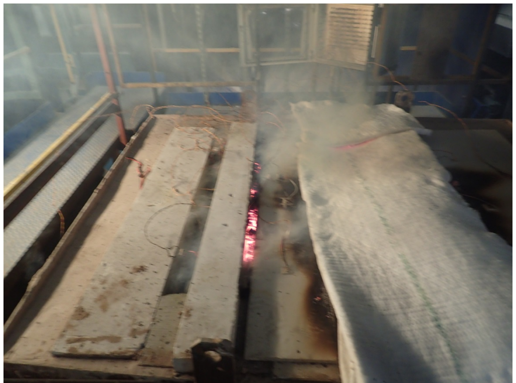
Integrity failure of Specimen D after a test duration of 48 minutes
