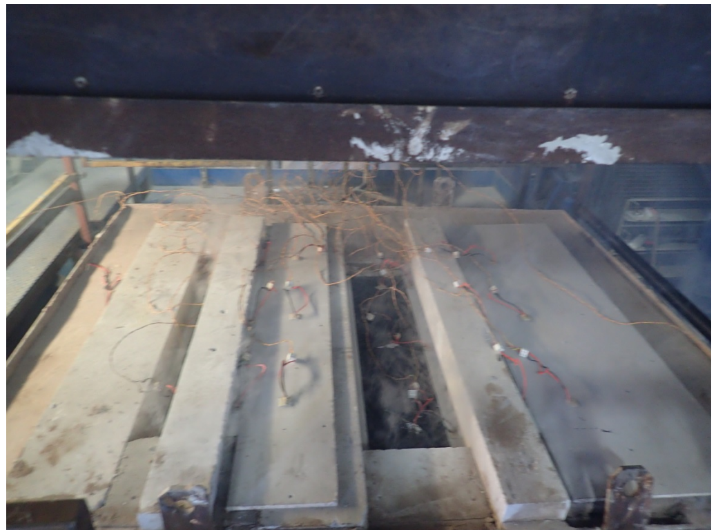
The unexposed face of the floor assembly after a test duration of 10 minutes
