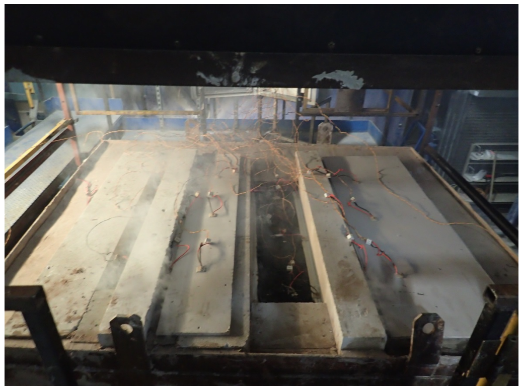
The unexposed face of the floor assembly after a test duration of 31 minutes
