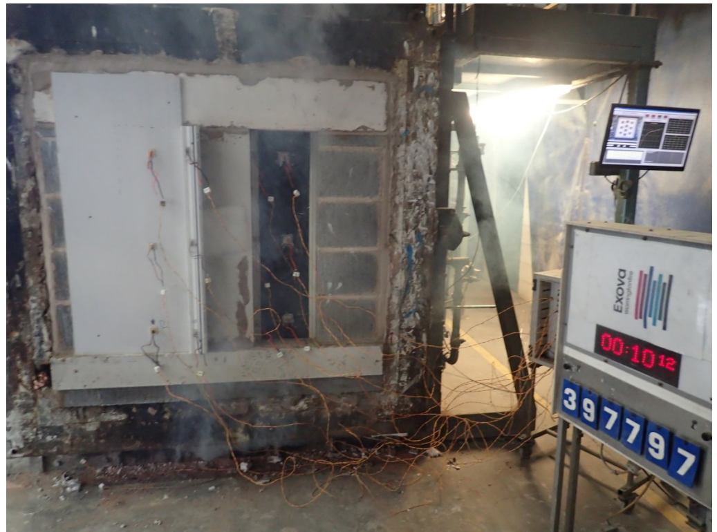
The unexposed face of the wall assembly after a test duration of 10 minutes
