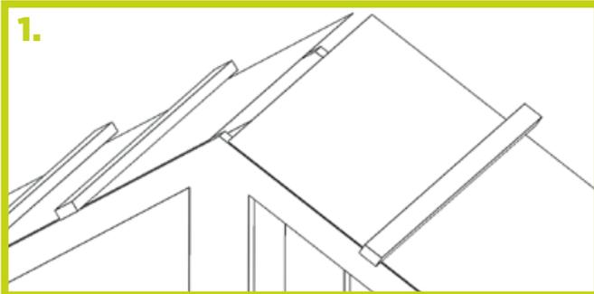
**1.** Apply the roofing underlay as normal practice leaving a gap of approximately 30mm short of the apex at both sides to allow for ventilation.
