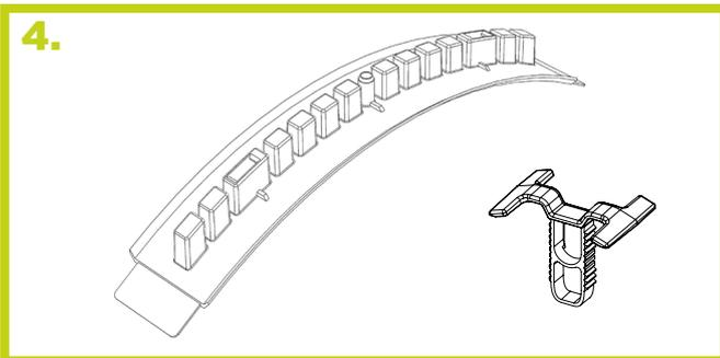
**4.** Place the ridge tiles along the ridge and join using the ridge union and clips provided.
