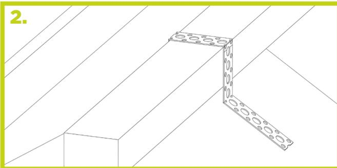
**2.** Span lengths of ridge batten along the roof apex and nail in place.
