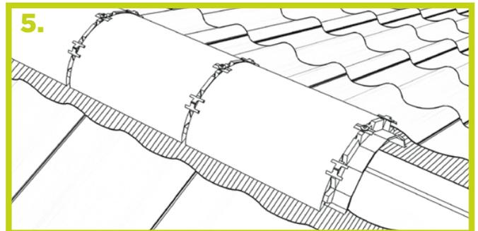
**5.** Position the adjacent ridge tile and then securely fix the screw and metal clamping plate through the top hole in the ridge union and into the ridge batten.
