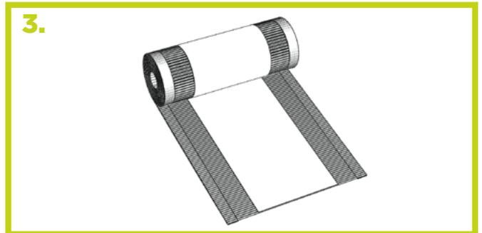
**3.** Lay out the roll evenly along the centre of the ridge batten and tack into position as the work proceeds using suitable roofing grade nails at rafter centre intervals. A minimum overlap of 100mm is required when starting a fresh roll along the ridge length.
