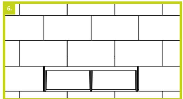
6. Now attach any manufacturer recommended tile clips onto the tile vent if required then continue with the main roof tile installation.
