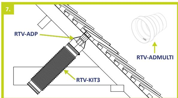
7. To connect the tile vent to a mechanical ventilation system or soil stack connect ductwork via the **RTV-ADP** 110mm duct adapter or via the **RTV-KIT3** 110mm Flexi-Pipe kit. The **RTV-ADMULTI** stepped duct adapter can also be used and cut to size to accommodate various duct diameters.
