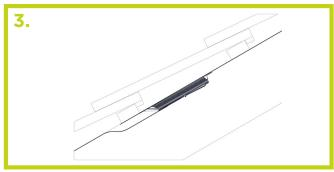
Push the lap vent down inside the joint ensuring the clips hook onto the outer face.
