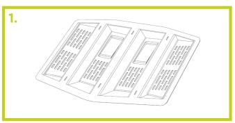
Ensure the lap vent is orientated with clips facing inwards to the roof space and the flat surface to roof.
