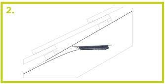
Insert the pointed edge of the lap vent into the gap between membrane/underlay overlap and then push flat towards roof line.
