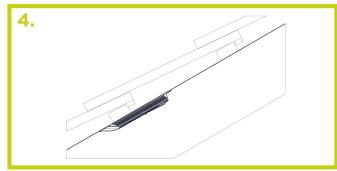
The lap vent is in the correct position when the clips are fully engaged onto the top edge of the membrane/underlay
