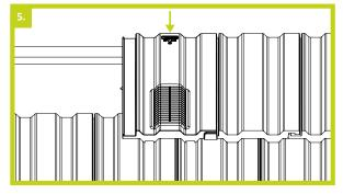
5. Use roof tile nails to secure the tile vent to the batten through the two raised hole areas. The nails will pierce through the plastic when hit to form the holes.
