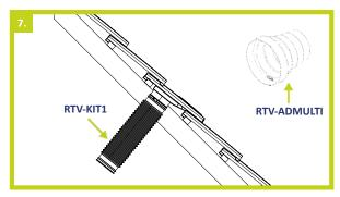
7. To connect the tile vent to a mechanical ventilation system or soil stack connect ductwork directly to the base of the tile vent or via the RTV-KIT1 110mm Flexi-Pipe kit. The RTV-ADMULTI stepped duct adapter can also be used and cut to size to accommodate various duct diameters.
