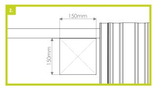
2. Mark out a rectangular area on the underlay just below the batten 150mm (W)  $\times$  150mm (H). Now mark a cross shape through the centre of the rectangular area to guide when cutting the underlay.
