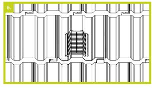
6. Now attach any manufacturer recommended tile clips onto the tile vent if required then continue with the main roof tile installation as before
