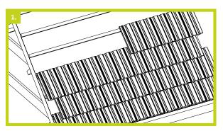
1. Install the roof tiles up to the tile space where the vent is required
