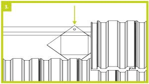
3. Cut along the diagonal cross shape lines then fold back the triangular flaps of the underlay to show the rectangular opening then fold the top tab tight against the batten and secure in place with a nail or staple.
