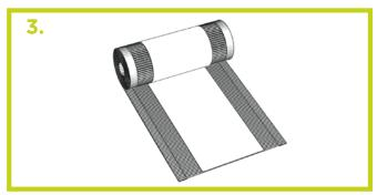
Lay out the roll evenly along the centre of the ridge batten and tack into position as the work proceeds using suitable roofing grade nails at rafter centre intervals. A minimum overlap of 100mm is required when starting a fresh roll along the ridge length.
