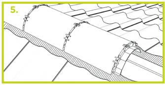
Position the adjacent ridge tile and then securely fix the screw and metal clamping plate through the top hole in the ridge union and into the ridge batten. a. Repeat the process as work ends.
