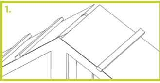
Apply the roofing underlay as normal practice leaving a gap of approximately 30mm short of the apex at both sides to allow for ventilation.
