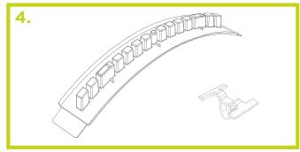
Place the ridge tiles along the ridge and join using the ridge union and clips provided. a. The ridge union clips are loosely clipped into the ridge union and offered up to the ridge tile. Once in position the clip can be pushed into place to contact ridge tile surface for a good fit.
