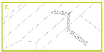
Span lengths of ridge batten along the roof apex and nail in place.
